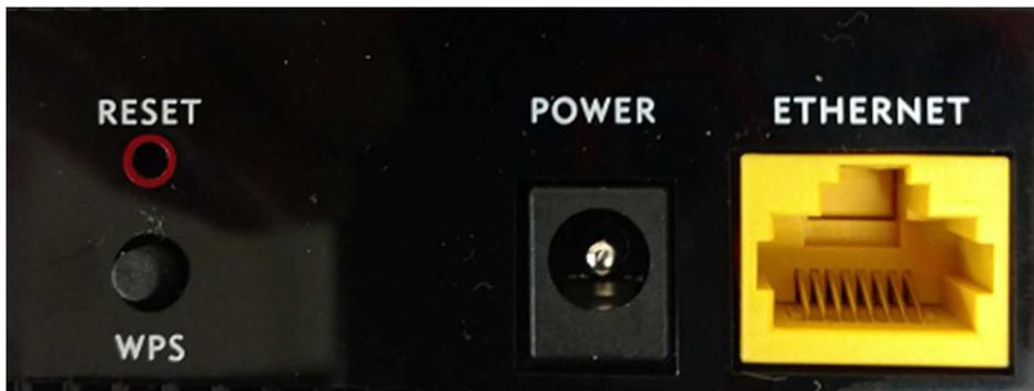
**Reset Button=** Under no circumstances should you insert anything into the reset button hole. This will result in a failure of services.
